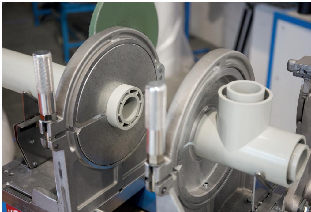
The AGRUCHEM Poly-Flo double containment piping system can be joined using time-saving simultaneous welding.
